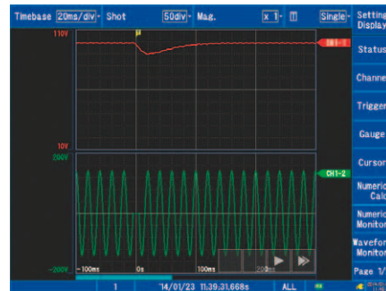
• Example of instrument recording the instantaneous waveform and RMS level waveform during a momentary outage of an AC power supply (using the MR8905)
