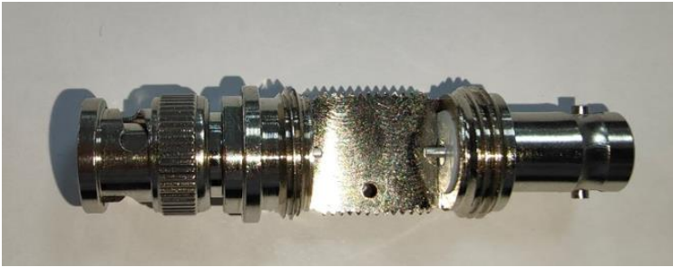
Picture 1: TBRFH7 RF housing components
