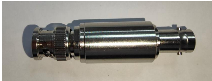
Picture 2: TBRFH7, assembled RF housing
