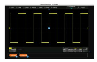
With the new embedded web server, users can control the oscilloscope from a simple web page. This provides wonderful remote troubleshooting and monitoring capabilities.
