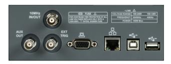
USB Host, USB Device (USBTMC), LAN (VXI-11, telnet, socket, web), Pass/Fail, Trigger Out, 10 MHz In/Out and VGA output
