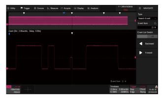
The SDS5000X can search events specified by the user in a frame. Events flagged by the Search can be recalled automatically using Navigate. It can also navigate by time (delay position) and history frames
