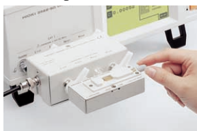
Example of connecting the 9262 and 9268 / 9269
