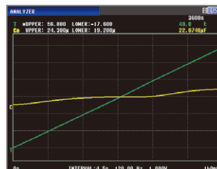
Interval measurement illustrating variation over time (Variation of laminated ceramic capacitor capacitance)
